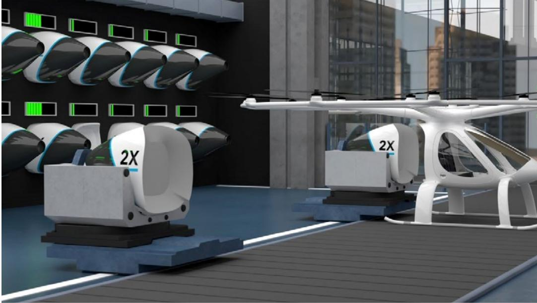
Figure 15 The Volocopter uses a battery swapping technique to maximize battery lifetime, and minimize turnaround time
