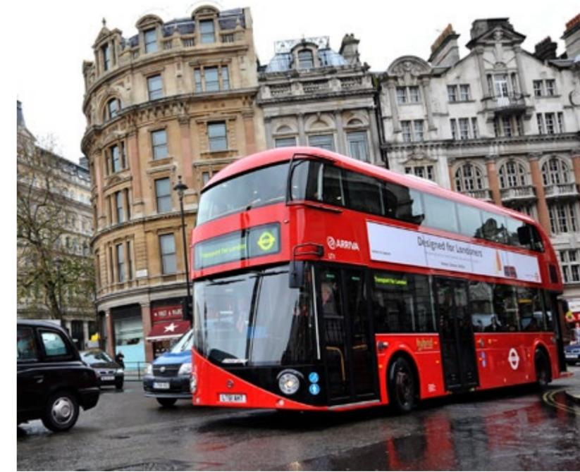
In London, hybrid electric double-decker buses equipped with IPT® Charge run in electric mode for more than 80% of the time over an operational day (20h), 7 days a week. Buses are equipped with 60 kWh batteries, and distance between charging options is 11 km.
