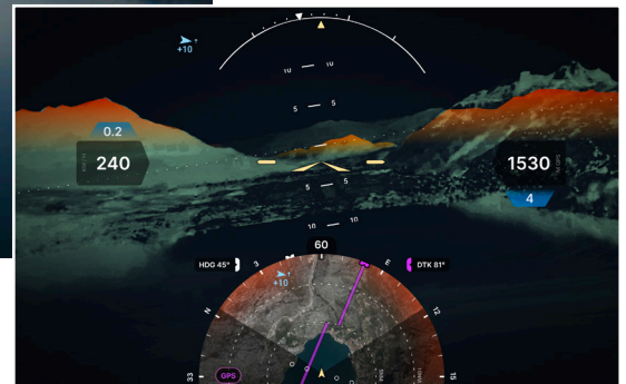
Conceptual view of a primary flight display with risk advisory, traffic collision, and landing guidance (daylight and night vision versions)
