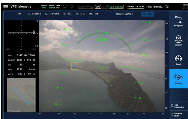
Examples of VXS at work, outputting the visual traffic detection information and visual landing guidance information on Daedalean's tablet app
